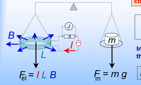
Weight of a test mass is compared with the force on a coil in a magnetic field.
